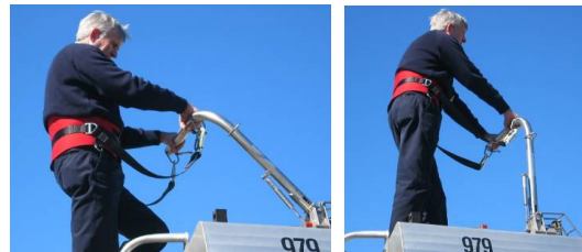
The transfer between the top of the ladder and the walkway using the TRAM
